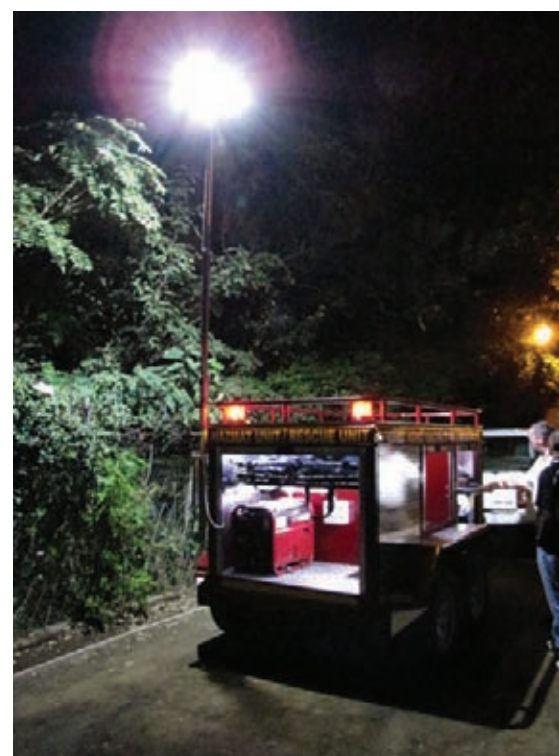
The hazmat trailer is fitted with a pneumatic extensible light mast for night operations
